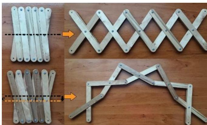
**Figure 11: Influence of Hinge Displacement on the Shape.**
