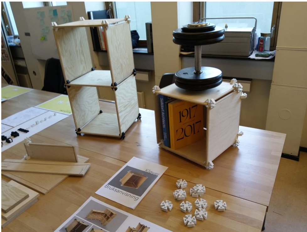
Fig. 4. Modular shelf system made by a group of six first-year students in two weeks.
