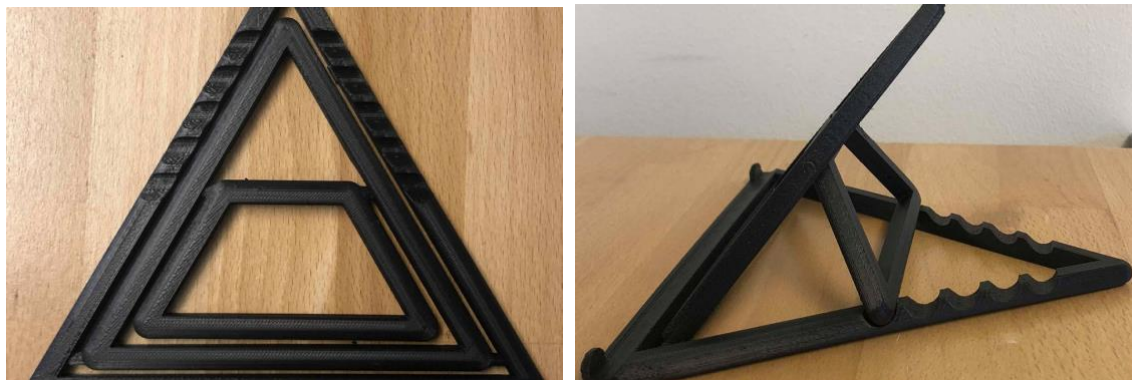
Fig.3: Example of a two week assignment inspired by affordances and disaffordances of 3D printers: holder for tablet -flat packed design is fast to print and without support material, while being easy to store and transport.
